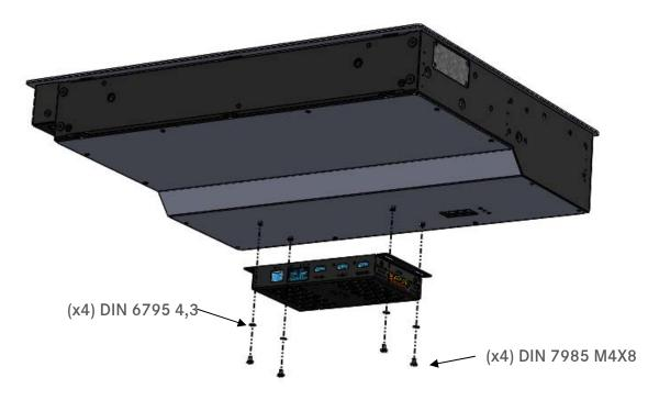
Dynamic Share/Loop is supplied with the necessary cables to be mounted under the Dynamic3. If desired, the Dynamic Share/Loop can be mounted outside Dynamic3 where the supplied cables harness allow.
