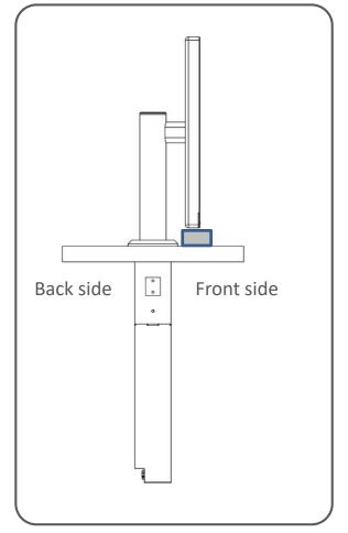
5 – Under the table: Pass the Protective and the Bracket ring trough the device.
