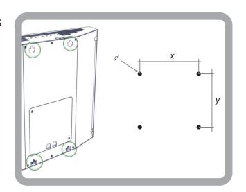
2.- To hang the monitor, place onto the wall and align it with the screws, making sure the monitor fits onto them, then slide it carefully down.
